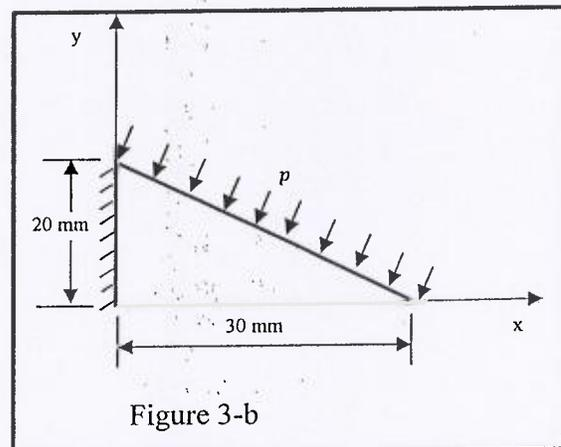
Show that for the plane stress condition, the  $2 \times 2$  matrix  $[k_{33}]$  is given by:
