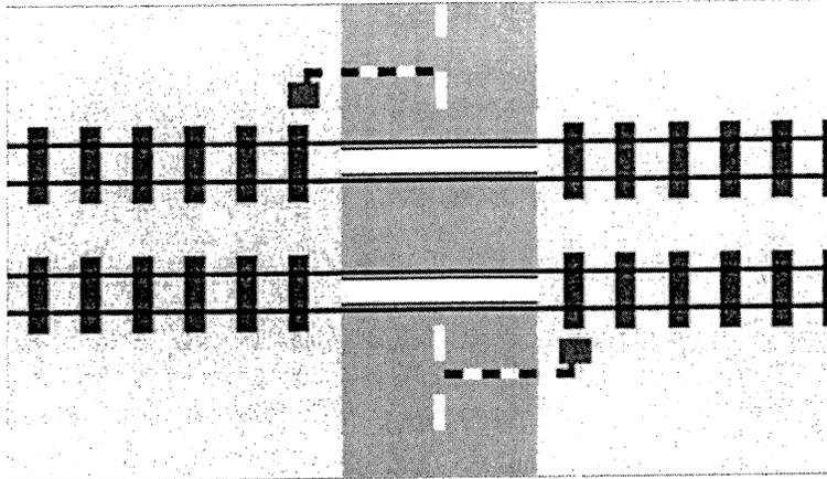
Also assume that the sensor to measure out-going train (train already passing the crossing) is located 20 m from the centre line of the road to trigger the lift of the gate. One wants the gate to be lifted as soon as the train has passed, consider the situations where two trains can come towards each other and pass through this railway crossing from both directions at same time.
