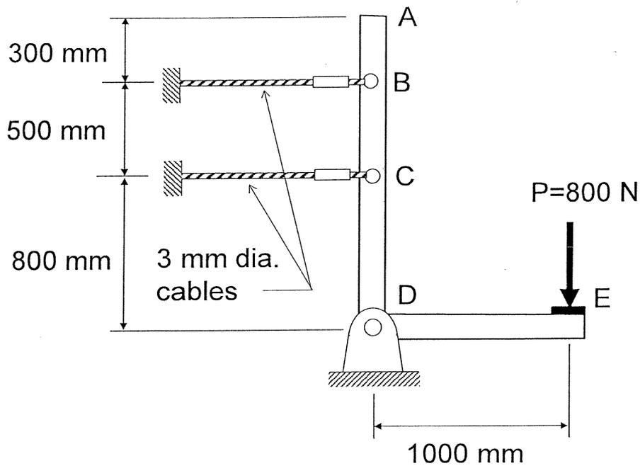
**Question 8** Determine the largest load  $P$  that can be applied to the truss structure below given [20 marks] that members AB and BC are made of 120 mm outside diameter hollow steel pipes with a 10 mm wall thickness. Both steel pipes are pinned at their ends.
