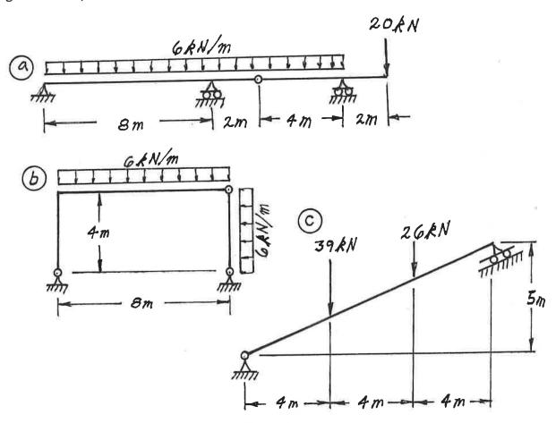
(18) 3. Calculate the vertical deflections at points B and D on the continuous beam shown below. EI<sub>0</sub> = 18000 kN.m<sup>2</sup>.
