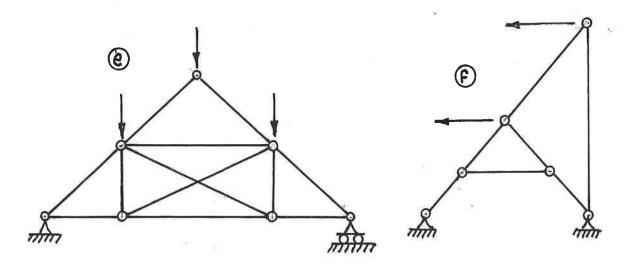
(18) 2. For each structure shown, compute the reactions and draw shear and bending moment diagrams (Choose one sign convention for plotting bending moments; use it consistently). For each member on the shear and bending moment diagrams, calculate and indicate the magnitudes of the maximum and minimum ordinates (Minimum ordinates are frequently negative values).
