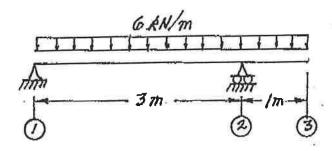
(18) 4. Use <u>Castigliano's theorem</u> (the least work theorem) to analyze the prismatic beam shown. Draw shear force and bending moment diagrams from point 1 to point 3. On both diagrams label the maximum and minimum ordinates. (Minimum ordinates are frequently negative values).
