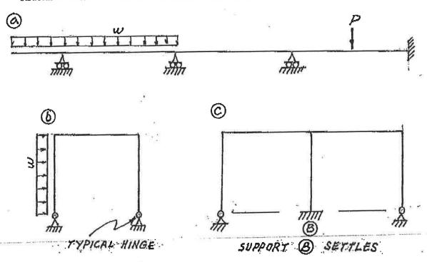
(8) 2. For each beam structure shown below, schematically show the influence line for the shear force immediately left of support (B). Note that structure a) is determinate and b) is indeterminate. Calculate and label the ordinate with the maximum absolute value on each influence line.
