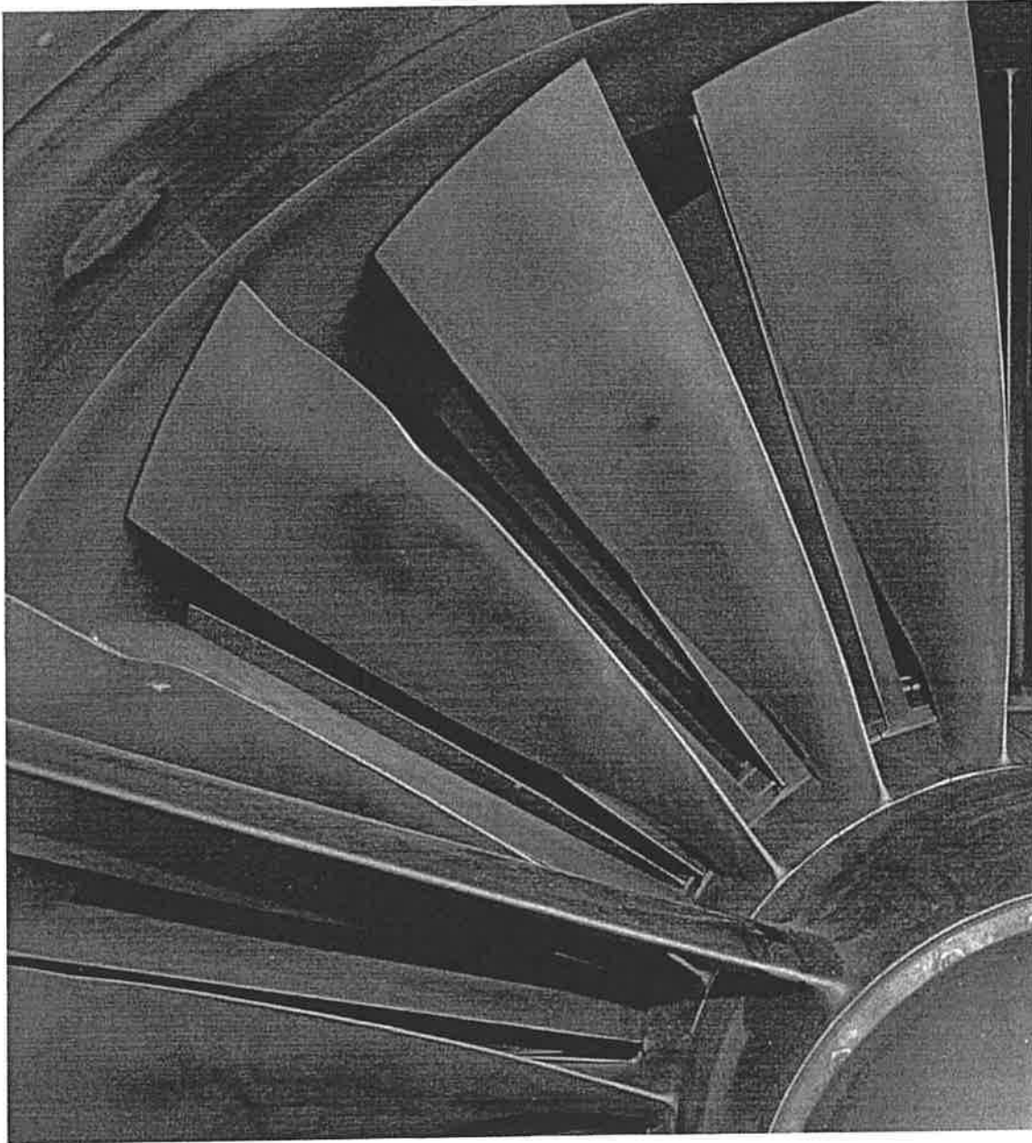
Rolls-Royce Olympus 593-610 first stage low pressure compressor blades
