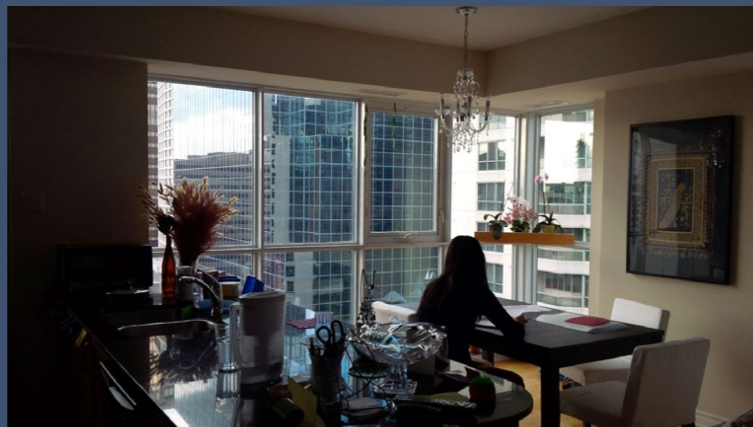
The outer perimeter near the windows of floor-to-ceiling glazed condominiums, like the unit depicted in this photograph, can become a source of discomfort during extremely cold and hot weather.
