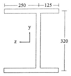
2. A thin-walled, cantilever beam supports two loads at its free end as shown below. Calculate the maximum bending and shear stresses at a section 500 mm away from the rigid support section. Assume the applied loads are acting at the shear center of the cross-section. (20 marks)
